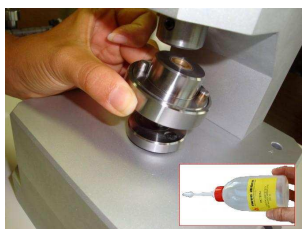
2 - Fitting of grinding disc support on DX75480 grinding machine.
